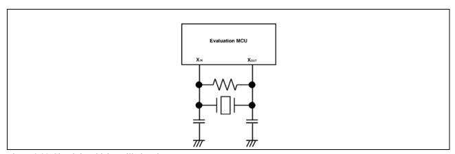
Figure 2.23 Circuit in which oscillation does not occur
